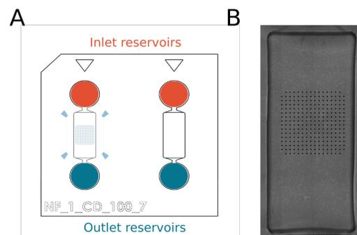
Figure 1. Microfluidic device for electrophysiological recording. (A) Schematic representation of a microfluidic chip (NF\_1\_CD\_100) coupled with MEA for electrophysiology recording. (B) Picture in brightfield light of a device with MEA.
